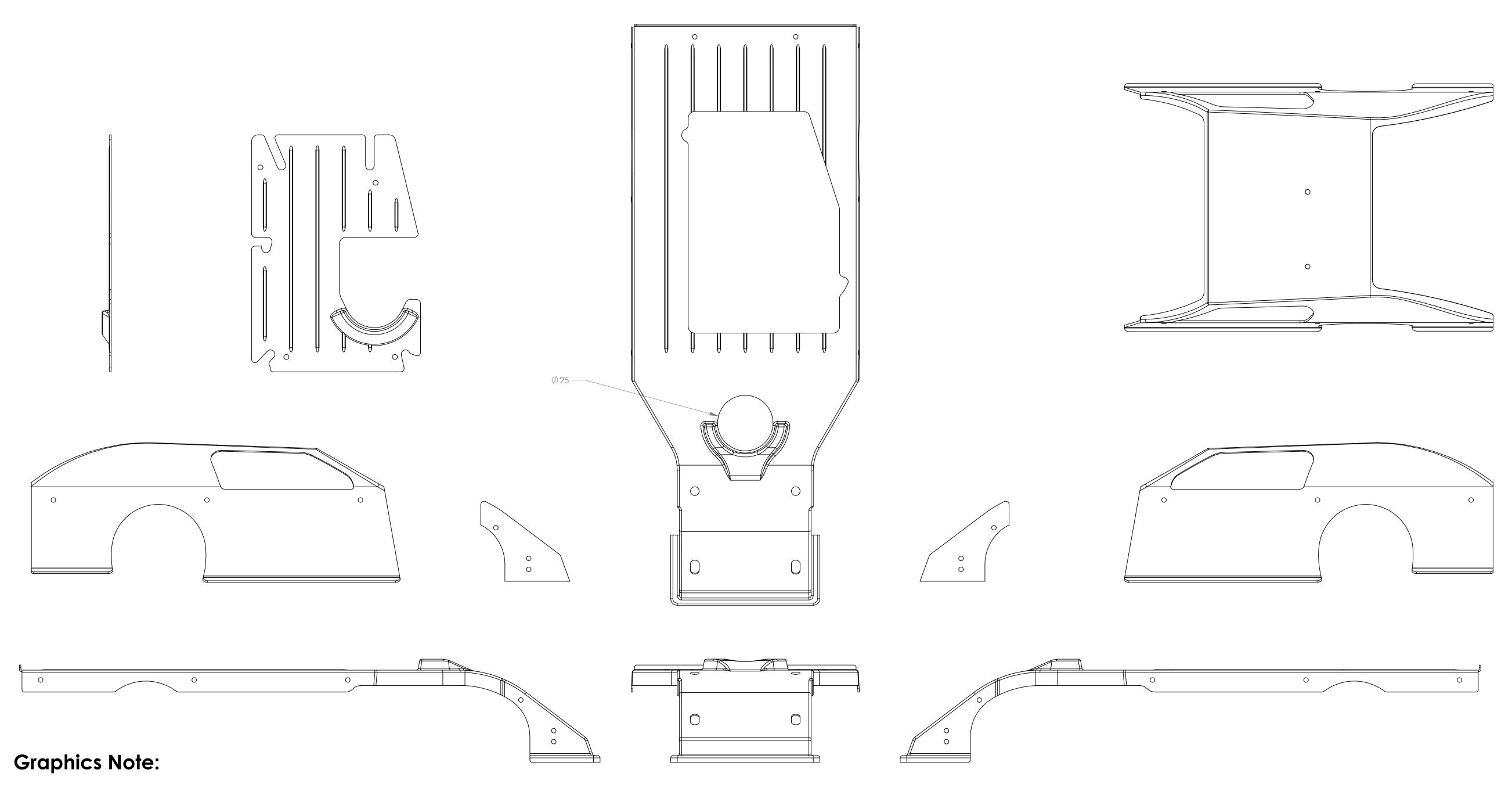
The images in this file are in the finished form and are not flat patterns of the parts so graphics may need to be adjusted to account for things like bends and other features that may exist on the body. We have added a hole dimension on the above image to ensure the file comes thru in 1:1 scale in your graphics system. 1 RC Racing, LLC is providing the files as a courtesy and is not responsible for any errors on graphics files produced from these images.
