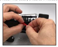
Step 1 - Plug Battery into Model
